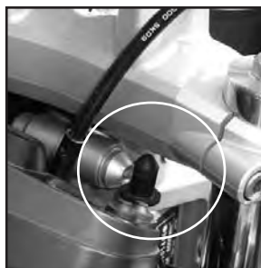
Rubber bushing may fall loose when releasing headlight stay.
