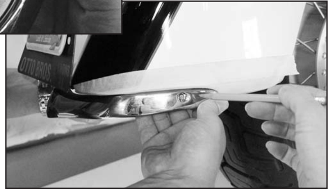
Figure 1. Tape Fender, Position Fender Tip, Mark Fender
