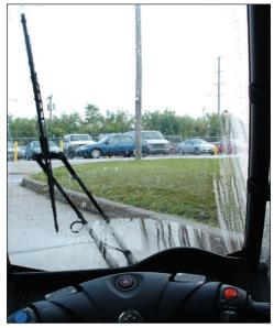
Award-winning Quantum hardcoating is used in many tough applications. Our Quantum hardcoated polycarbonate has withstood over one million windshield wipes on the windscreen of the fully enclosed Benelli Adiva scooter.
