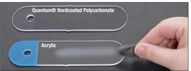
We use a steel wool scratch test to demonstrate the abrasion resistance of Quantum® hardcoated polycarbonate (top) against acrylic (bottom).
