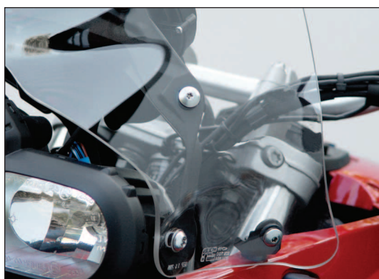
The lower contours add strength and rigidity.
