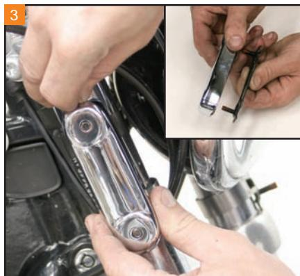
Now, put the mounting cup over the studs of the spider bracket.
