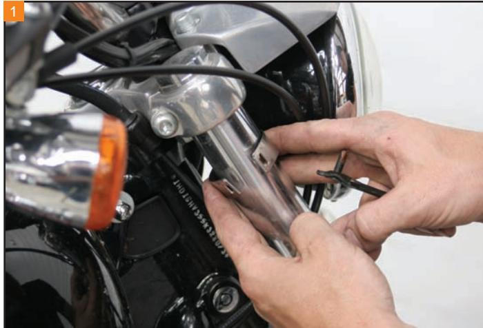
Install the clamp around the fork leg.
