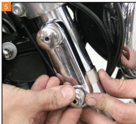
Put the small mounting spool on the lower stud.
