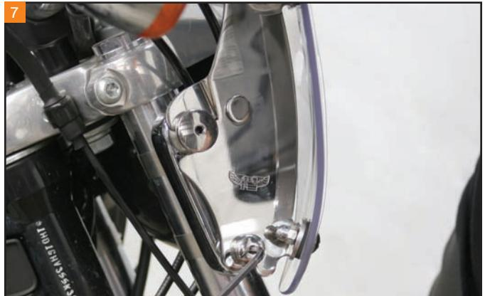
Tighten the hardware according to the instructions from National Cycle. Install and remove the windshield five different times. Finally, check the hardware and tighten if needed.
