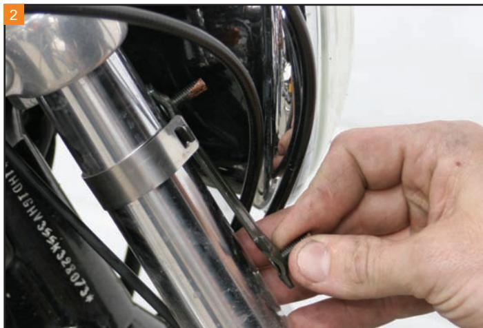
Attach the spider bracket to the fork clamp.
