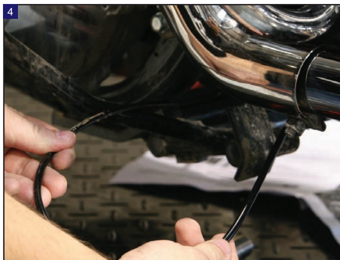
4 Route both diverter cables to the front right down tube.
