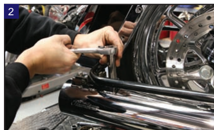
2 Slip the Peacemakers onto the exhaust header and tighten the rear hangar bolts and front exhaust clamp.
