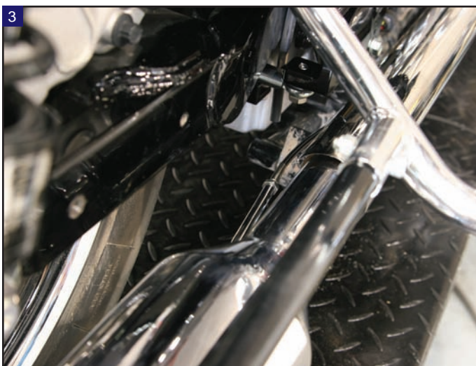
3 Note that the diverter cables are inside the mounted muffler.
