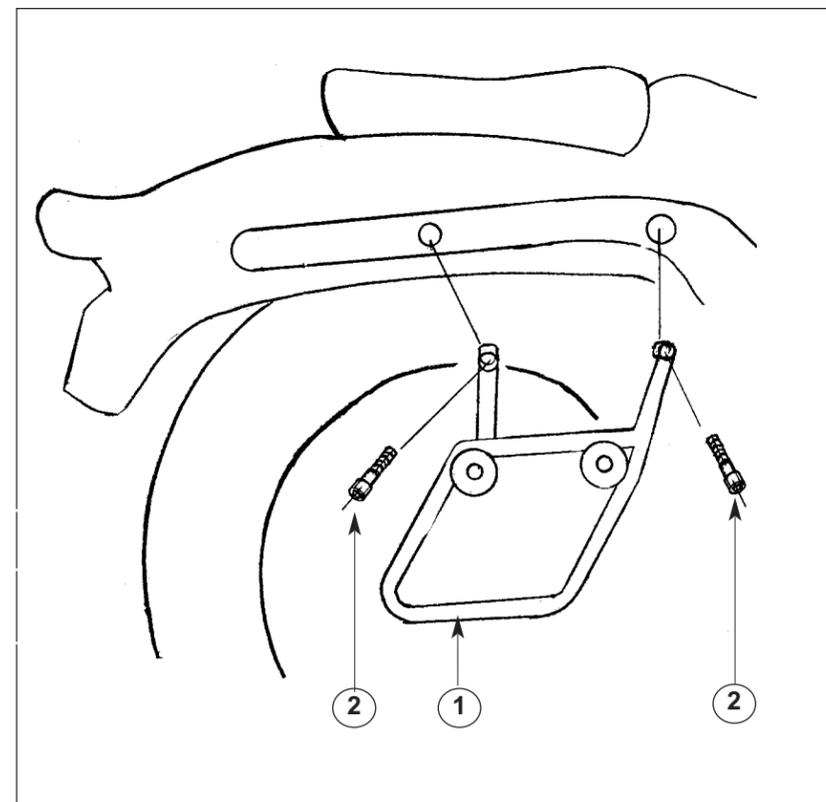
Remove the two forward screws from one Fender Strut (Wrench, 10mm).
