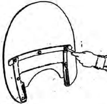
Use the screw removed from the front fork.
