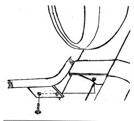
STEP 1 A. Use the M6 x 16 Screws to attach Light Bar Assembly under Lower Triple Clamp.
