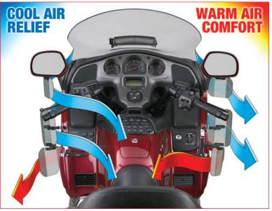
Wing Deflectors allow maximum **temperature control** of airflow toward or away from the rider. National Cycle's unique Swivel Ratchets allow each Deflector to be incrementally adjusted by hand for personalized temperature control. No tools required!
