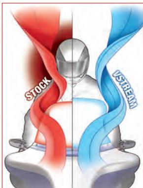
National Cycle's innovative **VStream® Windscreen** gets its name from the unique shape and dimensional contours designed and engineered into the windscreen. The patented "V" shape helps push the turbulent wind out and away from the side of the rider's head, producing a quieter and more comfortable riding experience for both the rider and the passenger.
