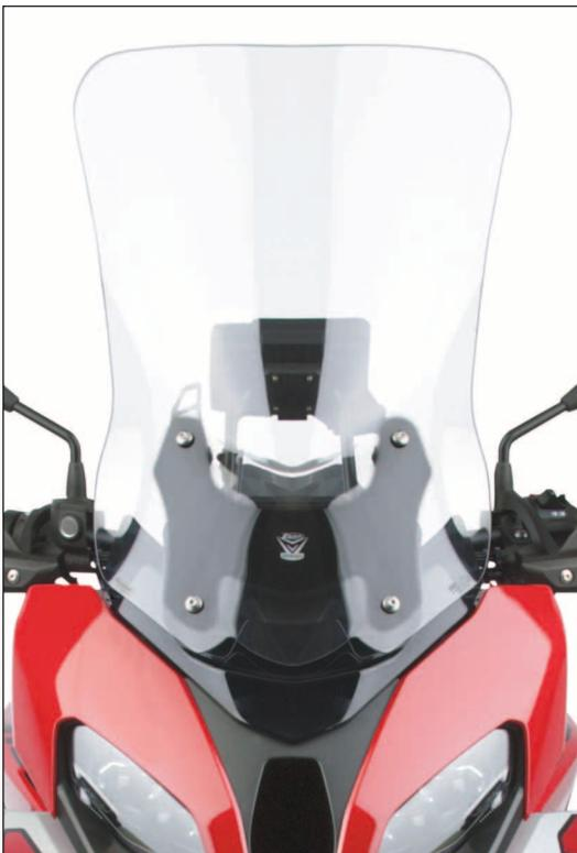
The Z2392-94 VStream® Windscreens mount easily using the OEM mount screws, and provide excellent wind protection and riding comfort.
