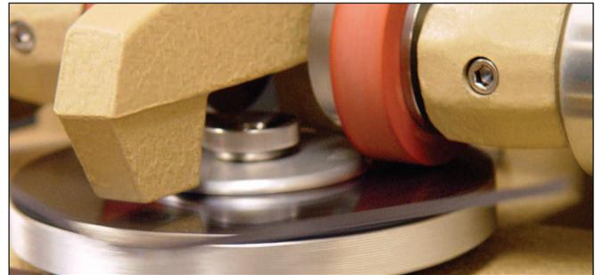
*Scientific laboratory monitoring and measurement instruments, like ZTechnik's Tabor 5130 Abraser, test the surface wear on both hardcoated and uncoated windshield materials.*
