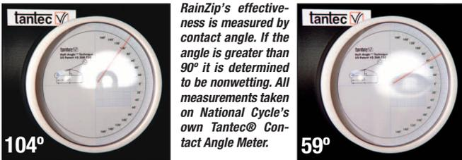
RainZip's effectiveness is measured by contact angle. If the angle is greater than 90° it is determined to be nonwetting. All measurements taken on National Cycle's own Tantec® Contact Angle Meter.
