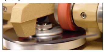
Scientific laboratory monitoring and measurement instruments, like ZTechnik's Tabor 5130 Abraser, test the surface wear on both hardcoated and uncoated windscreen materials.
