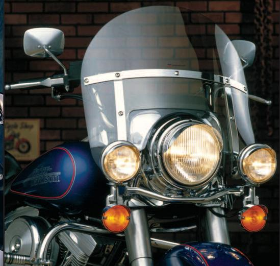
The **Beaded Heavy Duty™** is an authentic three-piece beaded construction. This timeless classic is available with a clear top and your choice of clear or black lower section and window. The traditional beaded edge is applied without glue to reduce yellowing and remain good looking for many years. The Beaded Heavy Duty is made from **FMR hardcoated Lexan® polycarbonate**.
