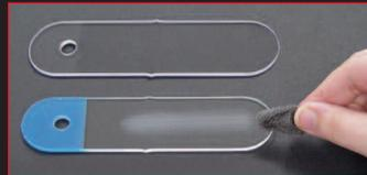
We use a steel wool scratch test to demonstrate the scratch resistance of Quantum hardcoated polycarbonate (top) against acrylic (bottom).
