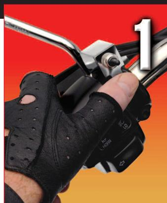
The handlebar-mounted toggle switch allows on-the-fly transitions between loud and quiet modes.
