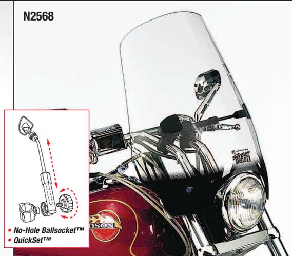
Riders will appreciate the **QuickSet™** mounting hardware that comes with the **Street Shield EX™**. The Street Shield EX is available in Light Tint (N2568) **High Impact Acrylic**.
