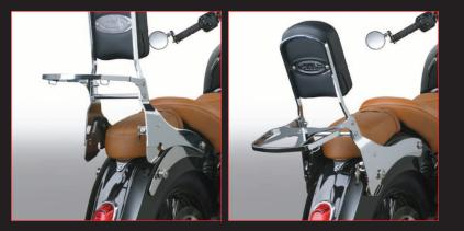
The **P9301 Backrest** can be mounted alone for carrying passengers. But with passengers, there is always extra gear to carry. Then you can simply add on the **P9302 Luggage Rack**.
