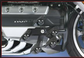
Optional Footpeg Mount Brackets provide 360° positioning for the footrest location most comfortable for the rider.
