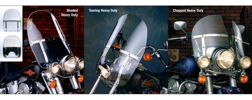
The **Beaded Heavy Duty<sup>TM</sup>** is an authentic threepiece beaded construction. This timeless classic is available with a clear top and your choice of clear or black lower section and window. The traditional beaded edge is applied without glue to reduce yellowing and remain good looking for many years. The Beaded Heavy Duty is made from **FMR hardcoated Lexan® polycarbonate**.
